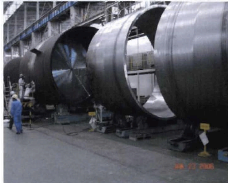
S/G 3A Lower and Middle Shell S/G 2A Balance Ring, Extension Ring, & Tubesheet
