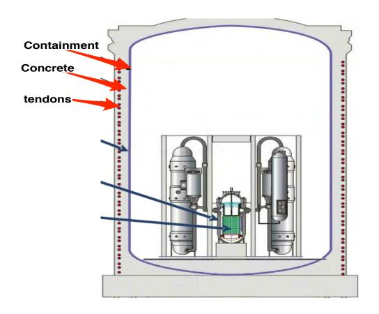
Since the tendons snapped on the Bellefonte Unit 1 Containment in 2009, both the NRC and TVA have been well aware that the containment at Bellefonte Unit 1 is severely degraded. First, in August 2009, a loud gunshot like noise was heard inside the containment. Finally, 100 days later, on December 10, 2009 Bellefonte acknowledged in LER 45559 that the Containment at Bellefonte Unit 1 had been compromised.
